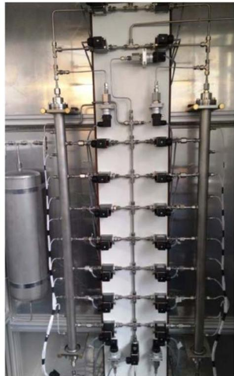
Fig 2: DR-PSA test rig
