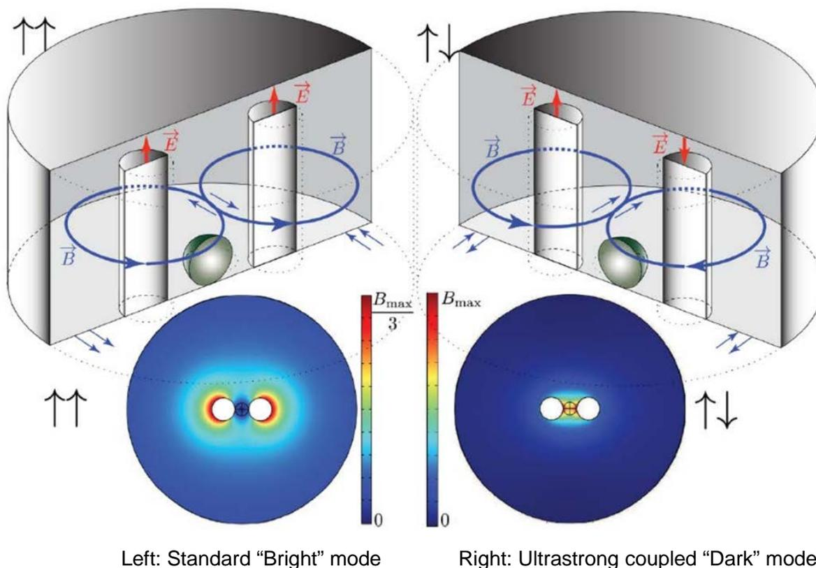
Example of a two-post version (basic building block of the 3D split-ring cavity lattice), implemented to create an ultrastrong hybrid quantum system between photons and magnons [3].
