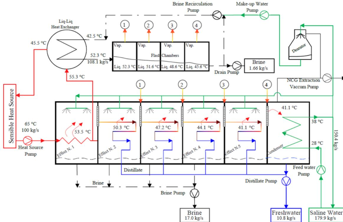
Figure 3: Flash Boosted MED System
