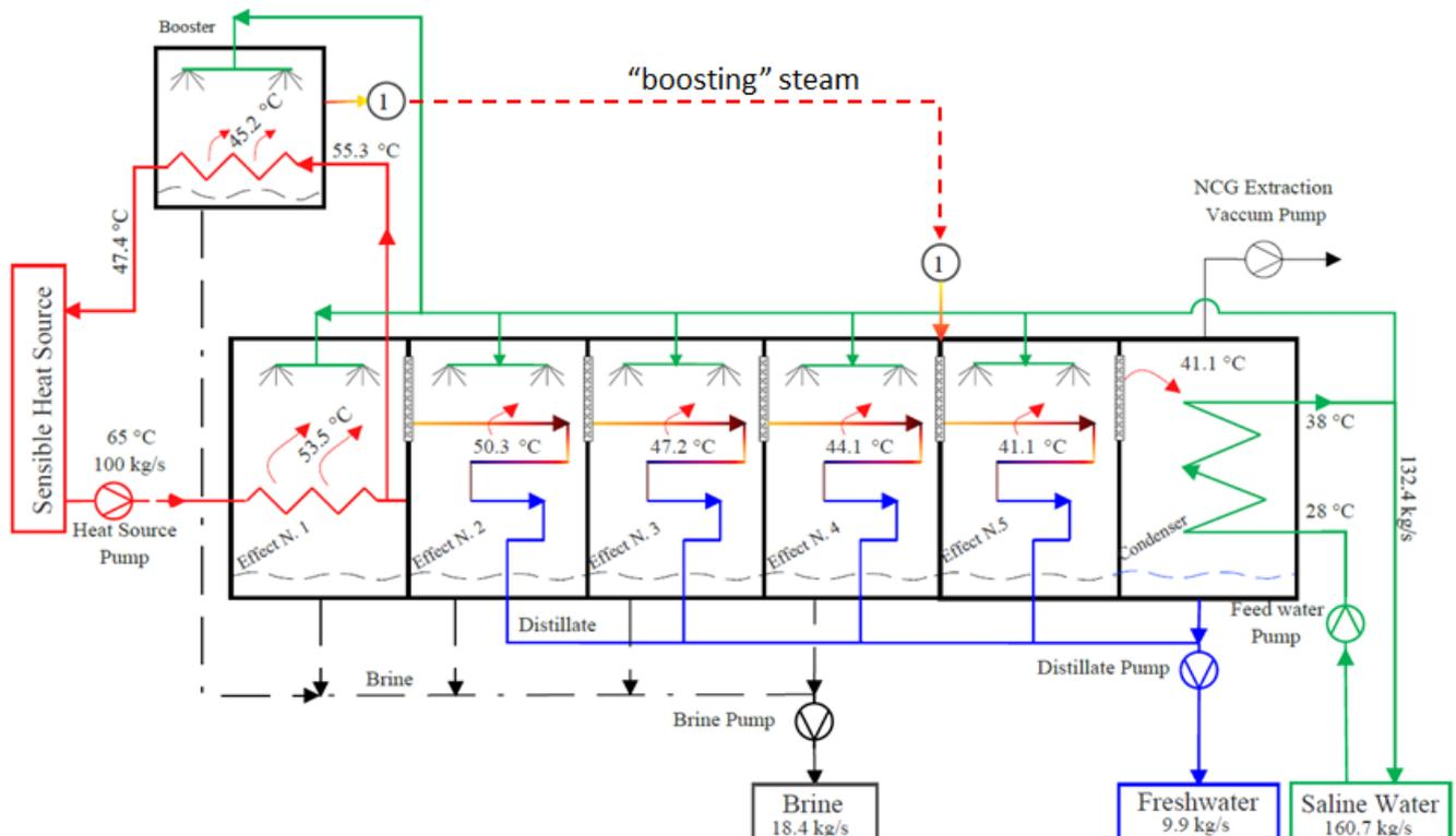
Figure 1: Steam Boosted MED System
