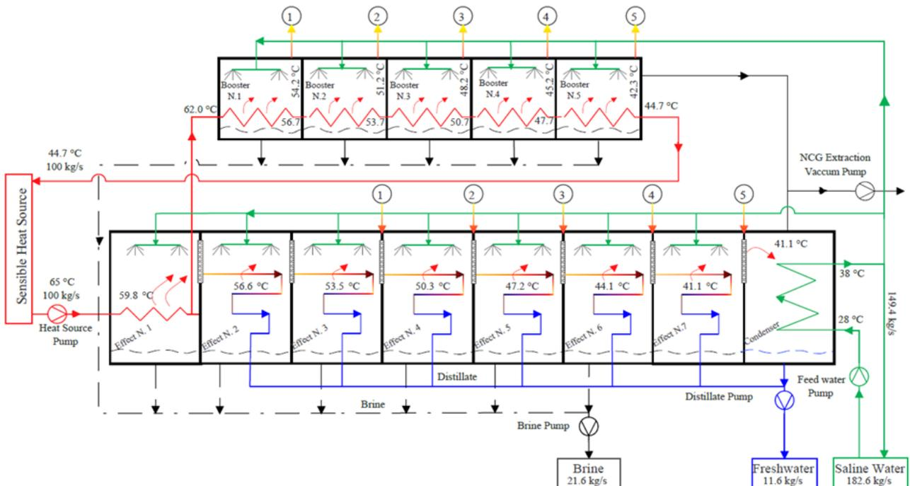
Figure 4: Distributed Boosted MED System
