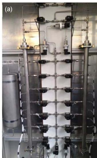
Fig 2: a) Pressure Swing Adsorption test rig
