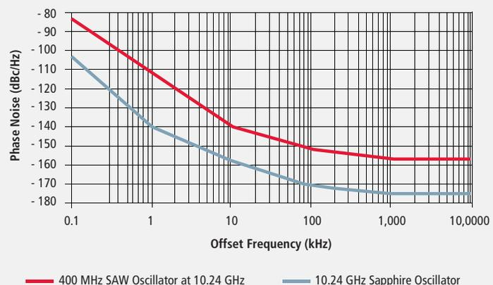
**Figure 2. Sapphire technology performance comparison: -20 dB better phase noise performance opens new doors for radar performance.**
